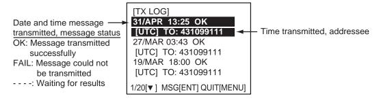
4. To view the contents of a message, select it with ▼ or ▲ then press the ENT key. Below is an example of a transmitted message. For an example of a received message, see section 1.8.2.
