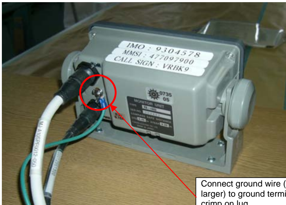
Fig. 8.2.2 Connection of AIS Display unit
