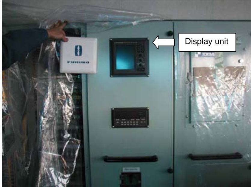
Fig. 11.3.1 Mounting of Display unit
