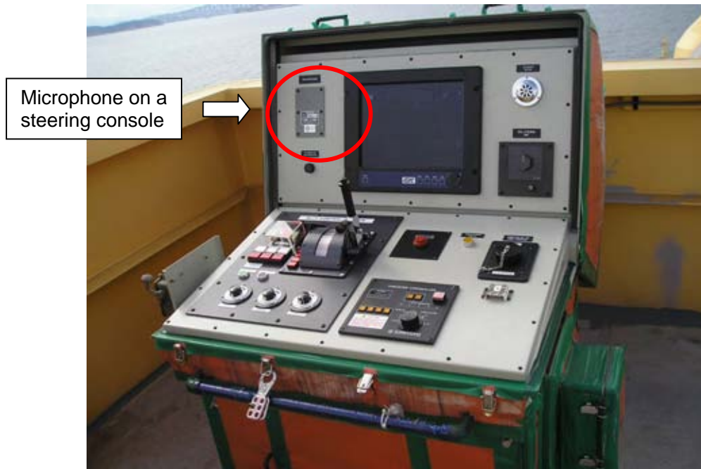
Fig. 9.2.7 Microphone on the steering stand of wing
