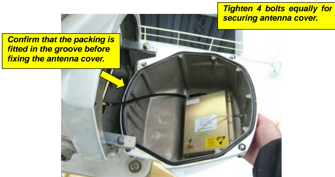
Fig. 1.2.9 Fixing antenna cover
