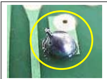
Bad example: Excess solder (causing vibration problem)
