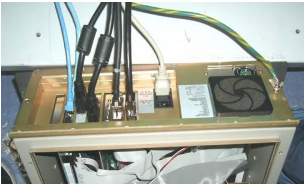
Fig. 2.1.5 Connection of processor unit
