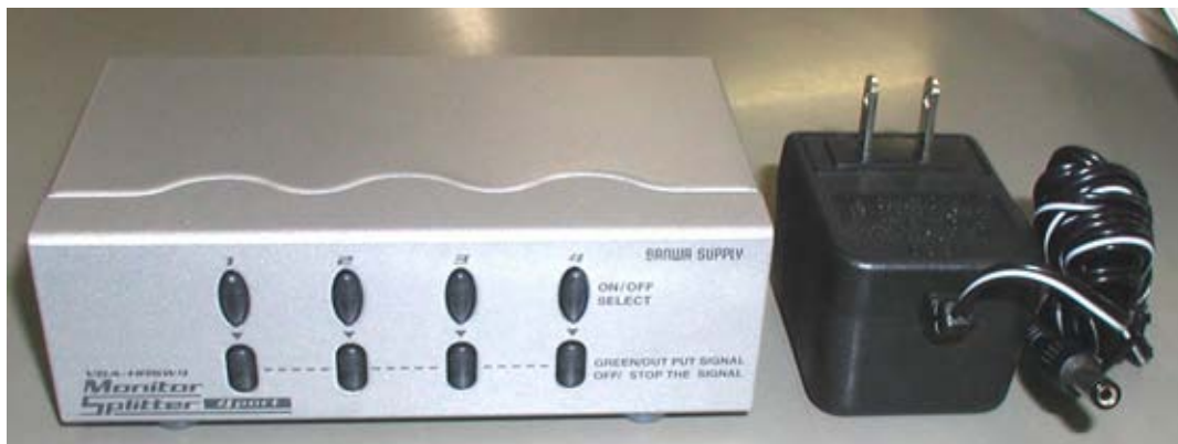
Fig. 2.3.2 RGB distributor "VGA-HRSW4"(SANWA Supply)
