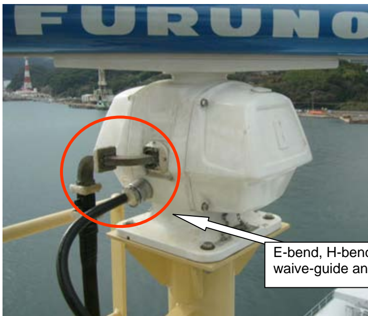
Fig. 1.2.16 Installation of wave-guide
