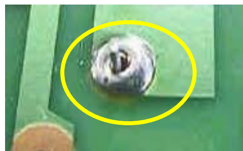
Bad example: Not enough temperature
