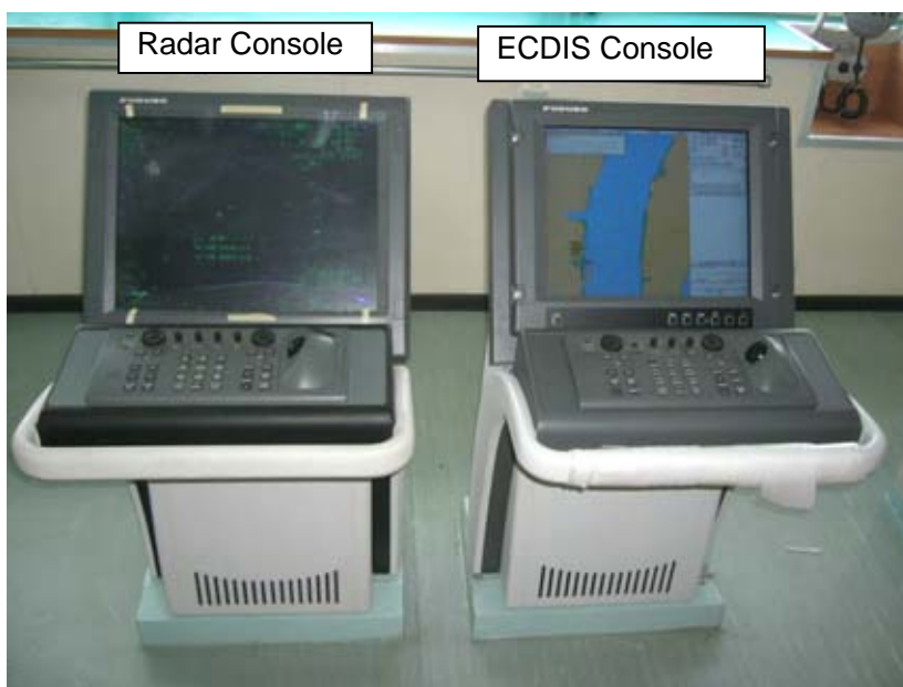
Fig. 2.1.2 Slim-type Radar and ECDIS console; ECN-001
