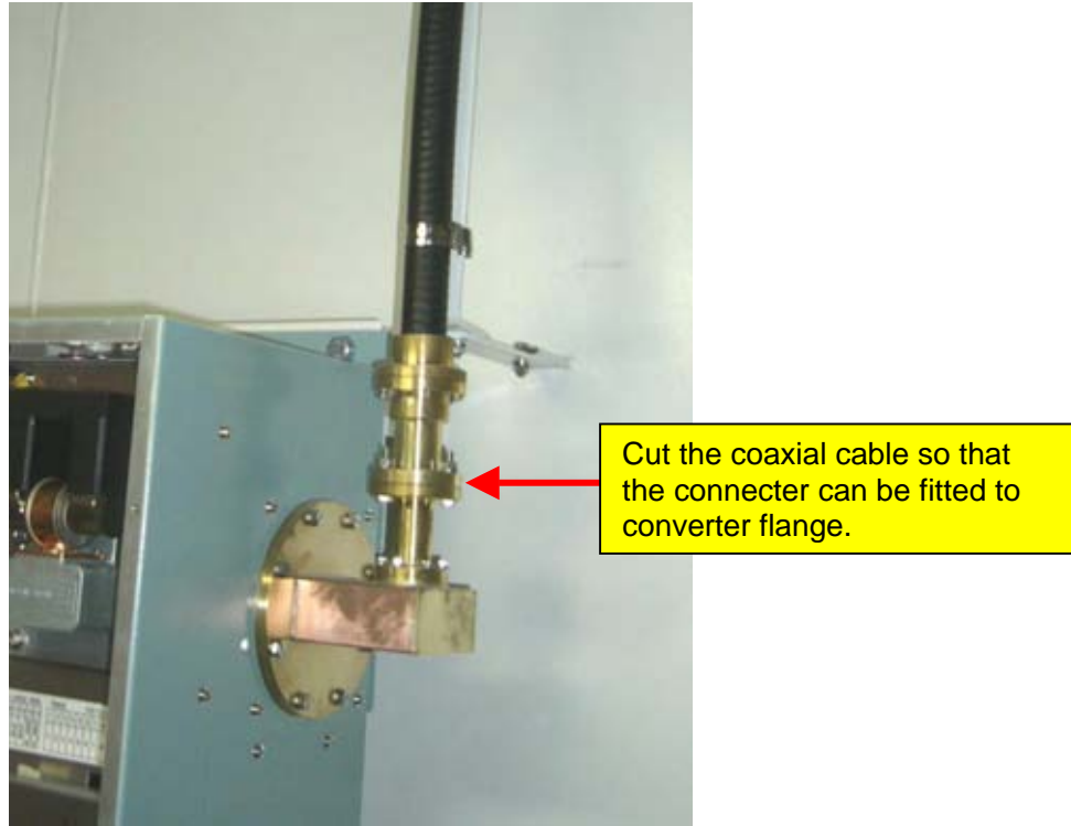
Fig. 1.3.15 Connection of coaxial cable
