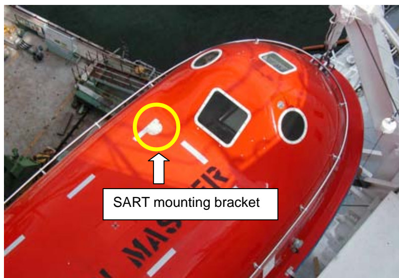
Fig. 10.1.2 Location of SART mounting bracket
