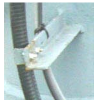
Fig. 1.3.9 Mounting of S-Band Radar: TR Down type antenna unit
