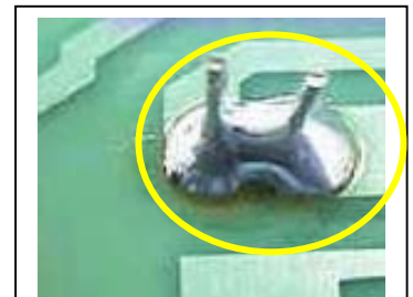
Bad example: Bridge to other contact
