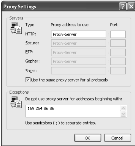
Figure 5.6: Use proxy server, unless the default IP address of the SB5006 service tool is requested.
