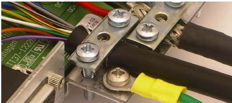
Figure 18 Fixation of the transceiver cable in TT-3616D.
