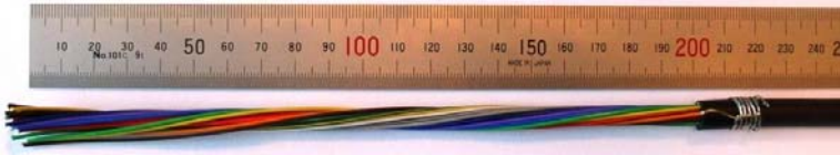
Figure 16 Transceiver cable preparation.
