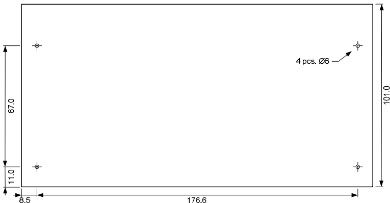
Figure 13 Drill template. All measures in mm.
