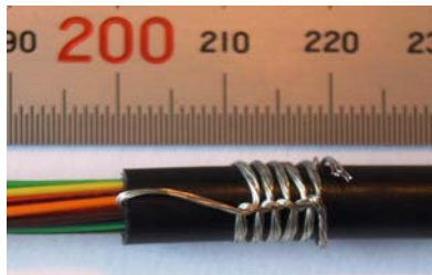
Figure 8 Preparation for grounding of the cable screen.
