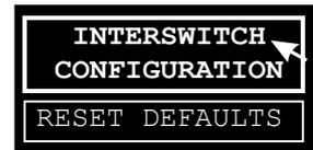
This will reveal a drop down menu (see example right) which gives the current transceiver/display configuration of the **whole system** with the **user's display channel(s)** highlighted in the left hand column.
