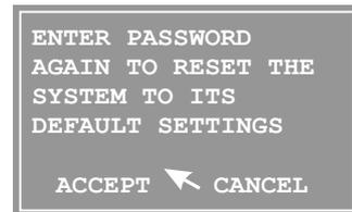
A left click on the CANCEL caption within the dialog box will close the dialog box and exit the reset facility without further action. The double entry of Manufacturer's password is used to confirm a positive and deliberate action to restore the system defaults. All user data is reset apart from the 'Hours Run' and 'Hours in Transmit' counters.
