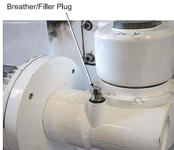
Figure 6.5 Zurrer Gearbox - Breather/Filler Plug
