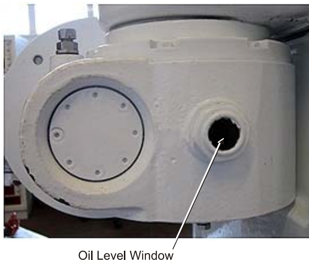
Figure 6.3 Zurrer Gearbox - Oil Level Window
