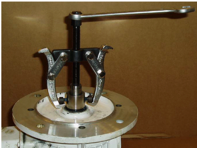
Figure 5.27 Removing Rehfluss coupling hub using Two Leg Puller
