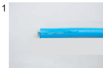
Expose inner vinyl sheath.
