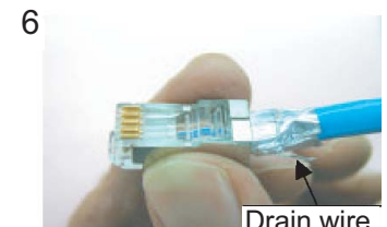
Insert the cable into the modular plug so that the folded part of the shield enters the modular plug. The drain wire must be on the tab side of the jack.
