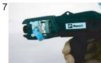
Using the special crimping tool MPT5-8 (PANDUIT CORP.), crimp the modular plug. Finally, check the plug visually.
