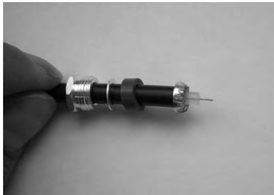
4) Slide clamp onto cable and fold back shield onto clamp.
