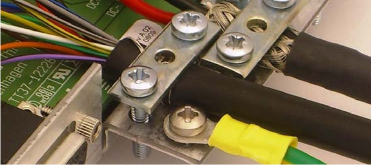
Figure 20 Fixation of the transceiver cable in TT-3616D.
