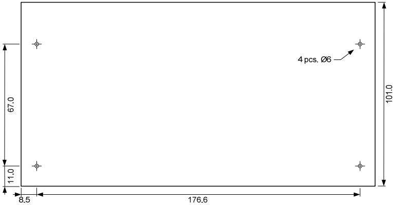
Figure 15 Drill template. All measures in mm.
