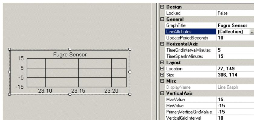
**Figure 3.14** Fugro Trim Sensor Line Graph
