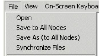
When you first access VisionMaster FT Configuration you must open the configuration file which matches the product type you are using. After opening the file, save the file as the default config file (named 'config.cfg') which will automatically be used by the VisionMaster FT system.
