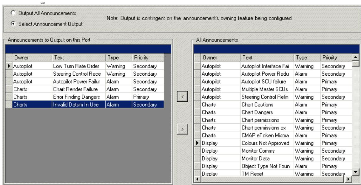
**Figure 1.160** I/O Configuration - select announcement output
