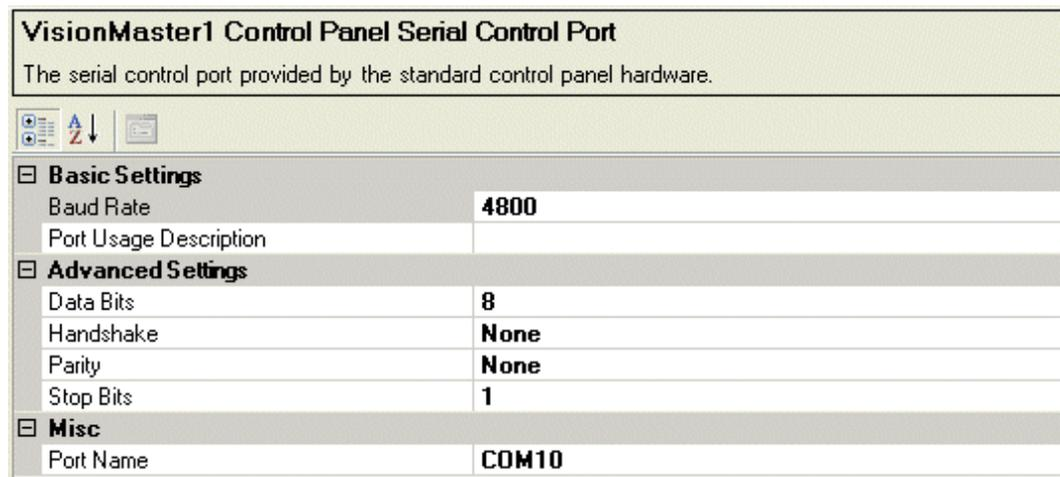
**Figure 1.64** Control Panel Serial Control Port Configuration Window
