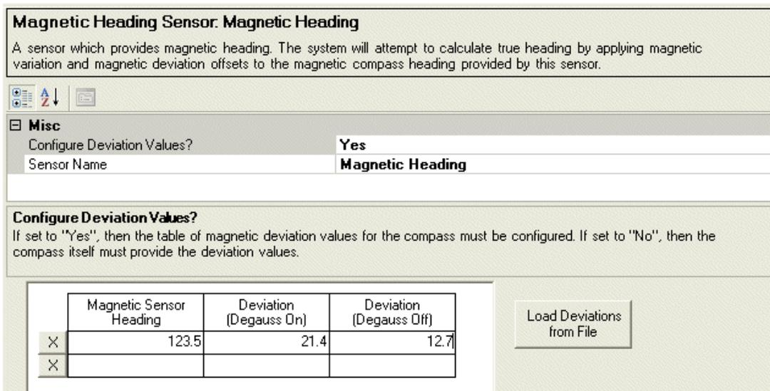
**Figure 1.94** Magnetic Heading Sensor with Deviation Values
