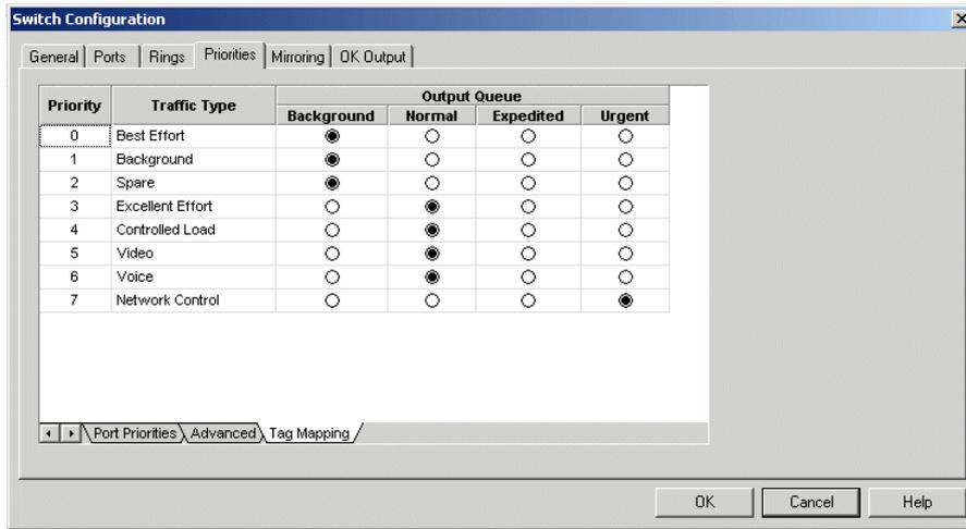
Figure C:28 9-Port Switch Configuration - Priorities - Tag Mapping
