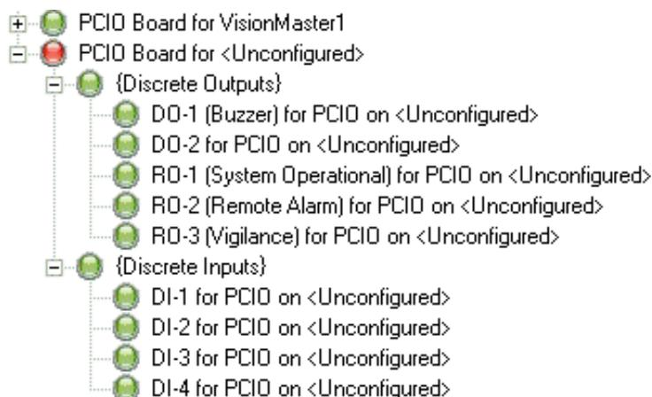
**Figure 1.39** Unconfigured PCIO Board - navigation tree
