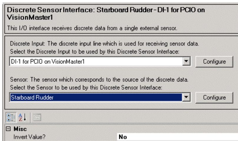
Figure 1.129 Discrete Sensor Interface
