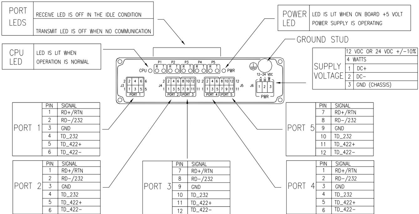
**Figure 2-2. Network Serial Interface Rear Panel**
