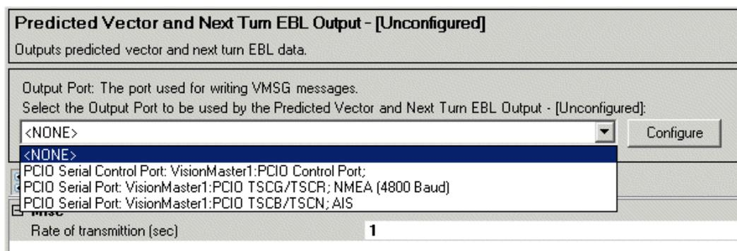
**Figure 1.90** Predicted Vector and Next Turn EBL output configuration
