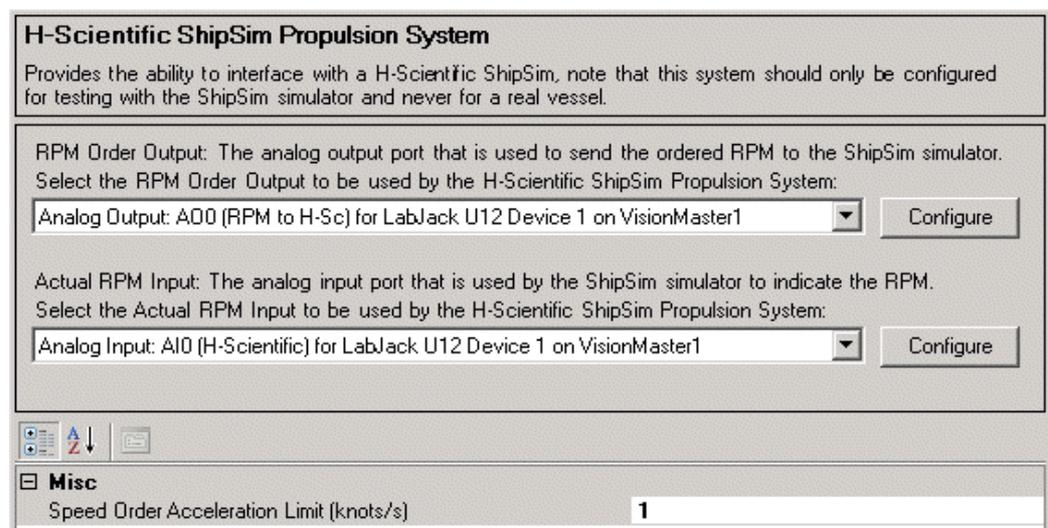
Figure 1.241 H-Scientific ShipSim Propulsion System
