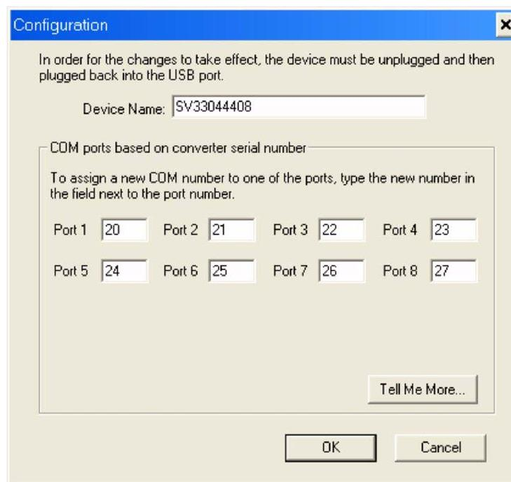
**Figure C:6** Edgeport Configuration for second Edgeport device
