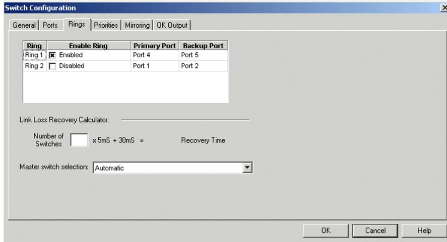
Figure C:17 5-Port Switch Configuration - Rings
