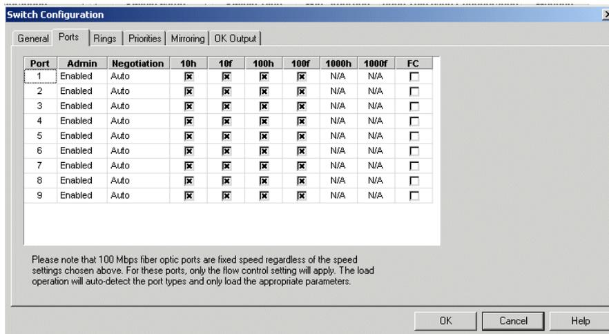
**Figure C:24** 9-Port Switch Configuration - Ports
