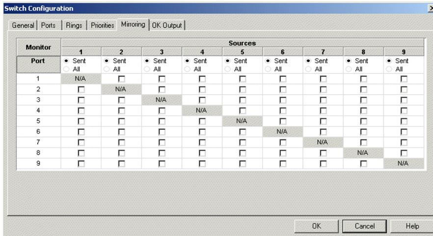
Figure C:29 9-Port Switch Configuration - Mirroring
