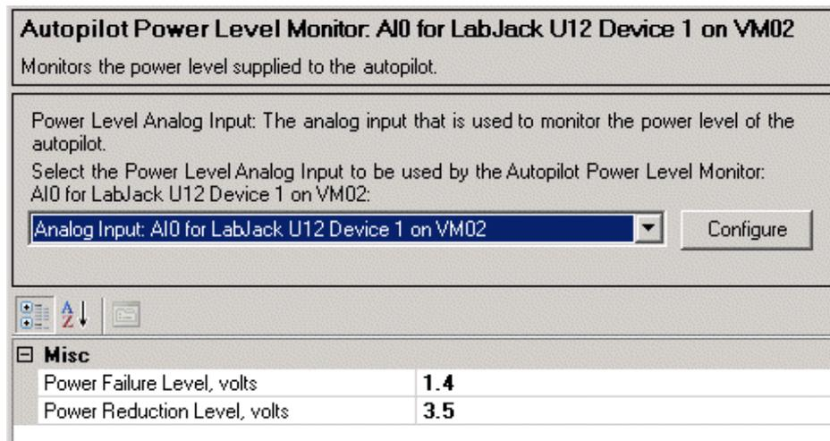
**Figure 1.208** Autopilot Power Level Monitor
