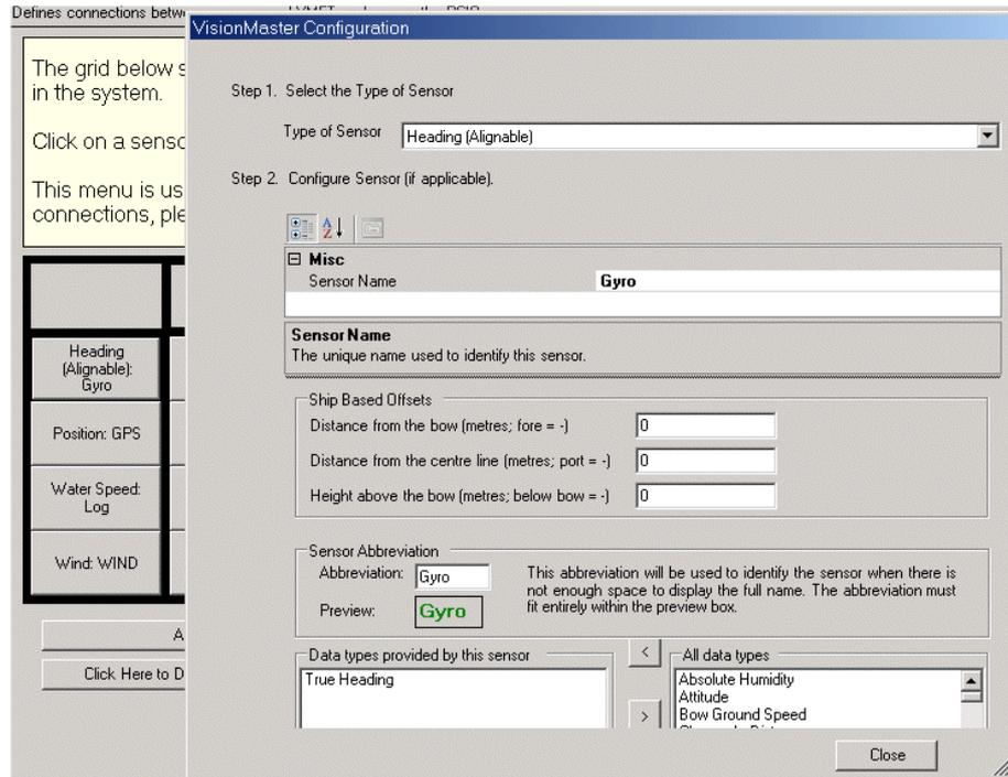
**Figure 1.14** Configuration Window for Heading Sensor
