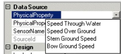
If an element has no data source configured the physical properties will show 'Generic Data' and the drop down list will include all data types.
