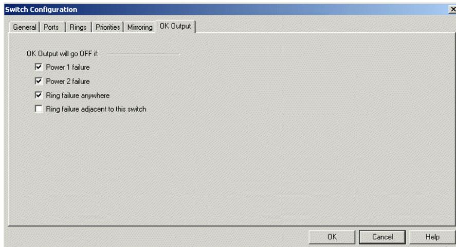
Figure C:30 9-Port Switch Configuration - OK Output
