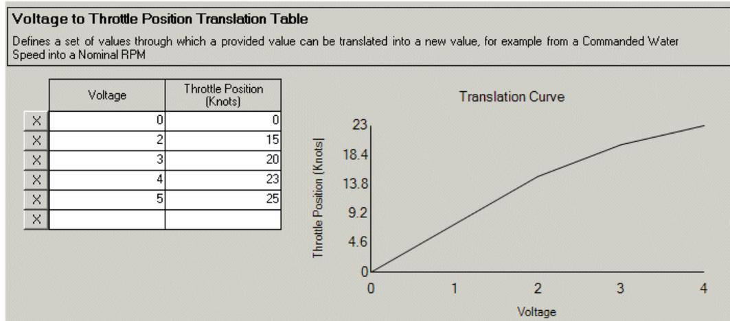
**Figure 1.233** Voltage to Throttle Position Translation Table - with five rows
