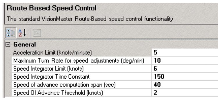
**Figure 1.224** Route Based Speed Control
