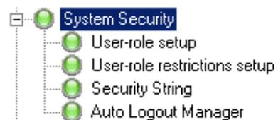
A security string is required when the VisionMaster system is multi-node. The security string also defines any optional features (such as 3D Vision or CCTV) that have been purchased by the customer.
