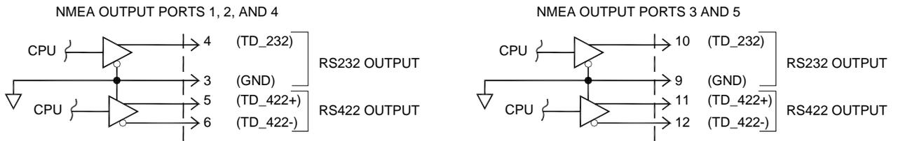
THE RS422 OUTPUTS MEET OR EXCEED T1A/RS422B AND ITU RECOMMENDATION V.11. THE OUTPUT HIGH VOLTAGE IS 2.4V MINIMUM AND 3.4V TYPICAL AT 20MA LOAD. DIFFERENTIAL OUTPUT IS 2.0V MINIMUM OR 3.1V TYPICAL WITH A 100 OHM LOAD.
