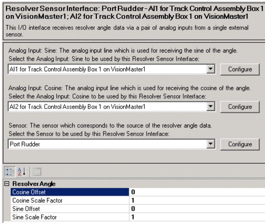
Figure 1.130 Resolver Sensor Interface
