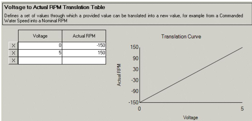
**Figure 1.240** Voltage to Actual RPM Translation Table
