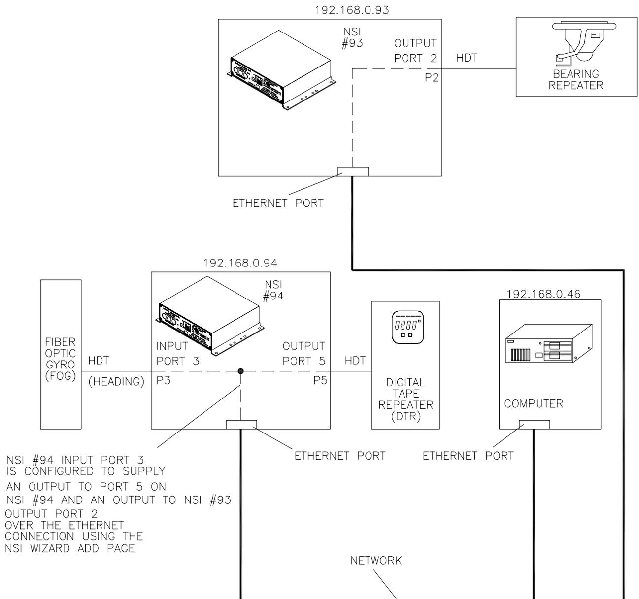
**Figure E-1. Sample Network Serial Interface Connection Block Diagram
