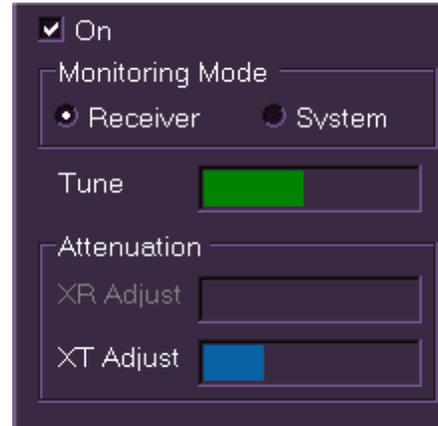
If any value is adjusted the new value is stored and restored both upon power up and when interswitching as Master to a transceiver. A different set of tune values are maintained for each transceiver.
