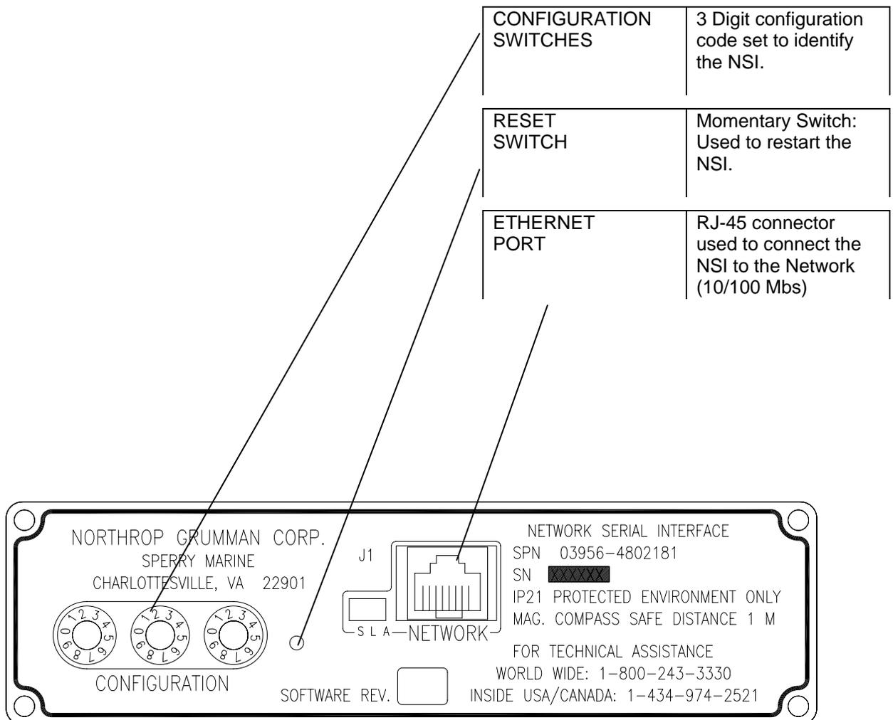
Figure 2-1. Network Serial Interface Front Panel
