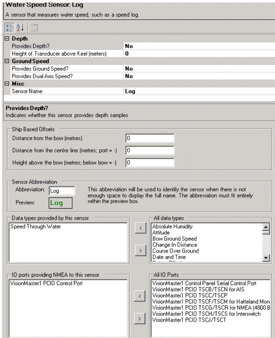
**Figure 1.96** Configuration Window for a Water Speed Sensor
