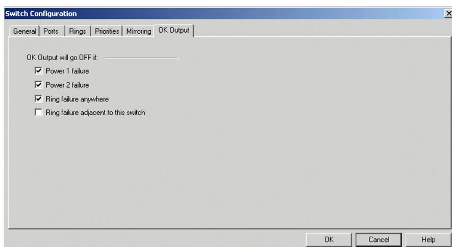
Figure C:22 5-Port Switch Configuration - OK Output
