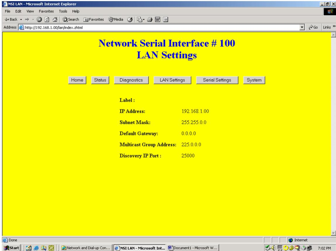
Figure 3-5. LAN Setting Page in Simple Mode
