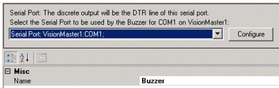
**Figure 1.77** Configuring a Serial Discrete Output
