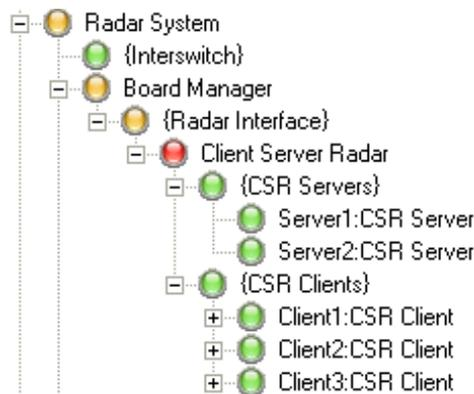
**Figure B.2** Client Server Radar Validation Error
