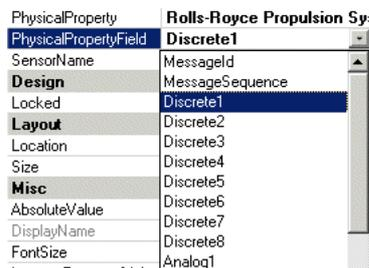
5. Click on the **SensorName** drop down list and select the sensor that corresponds to the message ID you wish to use. For example, if you need to display the 3rd analog value from the message identified as 0500 select **Analog3** as the physical property field and **Rolls-Royce Propulsion Sensor for message 05 sequence 0** as the sensor.
