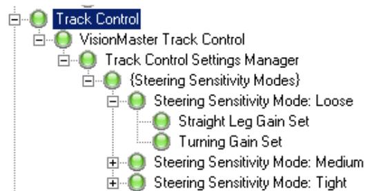
This section also includes instructions on configuring VisionMaster track control settings to correspond to existing track control settings from a legacy VMS (Voyage Management System). See *Section 8.10.18.2 Configuring VMFT Track Control Settings from VMS*.
