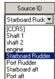
2. If CCRS is the source ID select the required data type. When a specific sensor source ID is selected, the Data Type and Data Field are automatically populated with the data type and value provided by this sensor, for example, 'Engine RPM' for Engine Sensor or 'Rudder Angle' for Port/Starboard Rudder.
