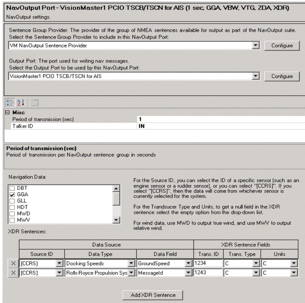
**Figure 1.137** Nav Output Configuration
