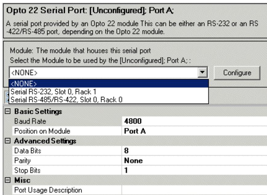
**Figure 1.67** Opto 22 Serial Port Configuration Window
