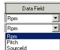
4. The XDR Sentence Fields define the content of the transducer ID, the transducer type, and the units of measure fields, as described above (where the XDR sentence format was defined). Any values may be used for the transducer ID. Only legally defined values may be selected for the transducer type and the units.
