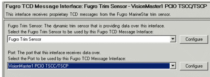
**Figure 1.105** External Sensors Fugro Interface Configured
