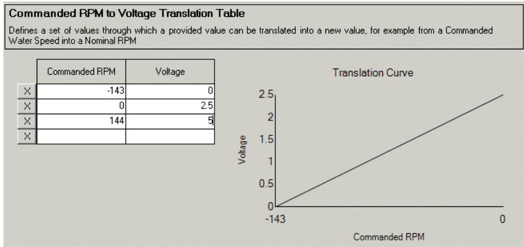
**Figure 1.239** Commanded RPM to Voltage Translation Table
