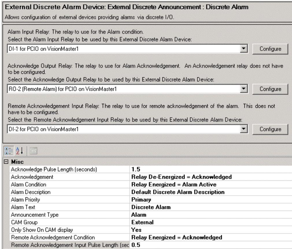
**Figure 1.162** External Discrete Alarm Device Configuration
