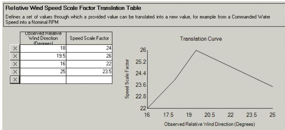
**Figure 1.99** Relative Wind Speed Scale Factor Translation Table
