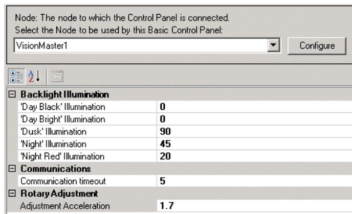
**Figure 1.42** Basic Control Panel Configuration
