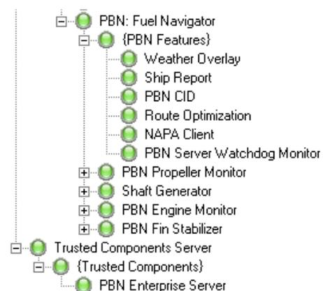
For ship reporting from other VisionMaster subsystems data is retrieved to populate ship reports. The PBN Fuel Navigator sends the XML based ship reports to the PBN Enterprise Server where they are transferred to the shore based reporting system via the ship's on board satellite communication system.
