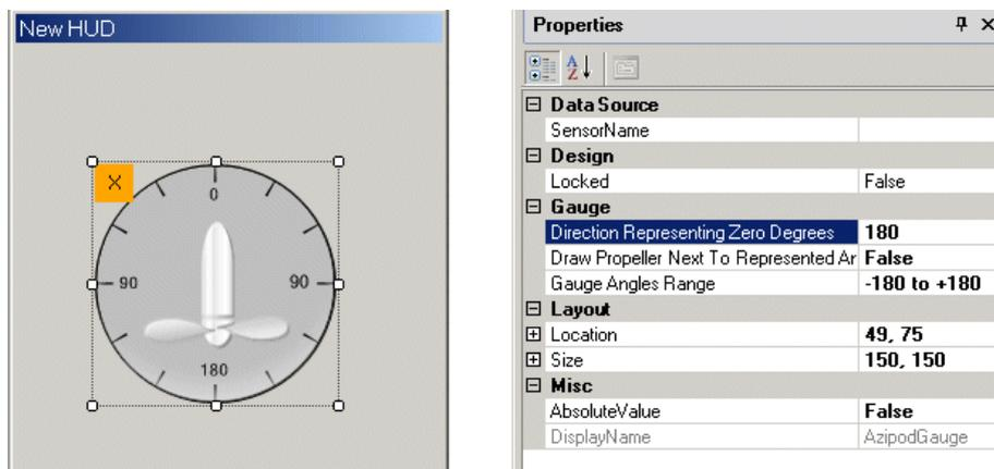
**Figure 3.12** Azipod Gauge Reversed for Aft Facing Display
