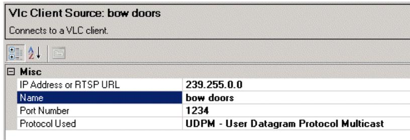
**Figure 1.71** Vlc Client Source Configured
